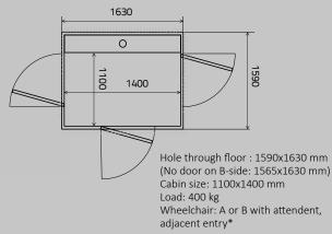
Wheelchair Type A and B according to EN 12183/EN 12184.
